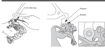
Bracket spindle Tightening torque: 8 - 10 N·m {70 - 86 in. lbs.}
